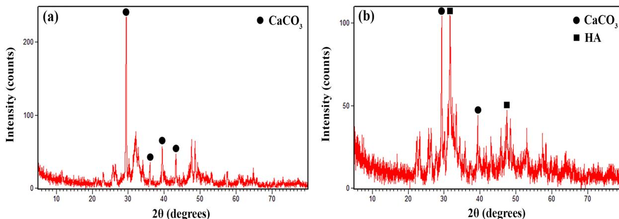
Fig. 1. a) XRD patterns of eggshell powder and b) synthesized hydroxyapatite.
