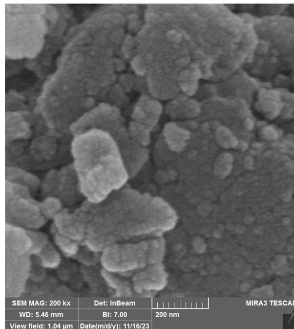
Fig. 3. Scanning electron microscopy image of nano-hydroxyapatite powder made from eggshells.
