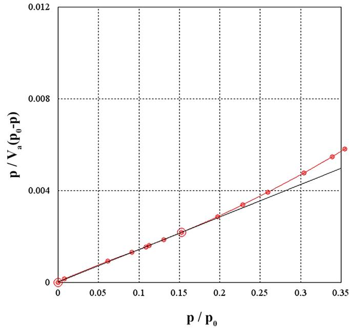
Fig. 2. BET curve of hydroxyapatite sample.
