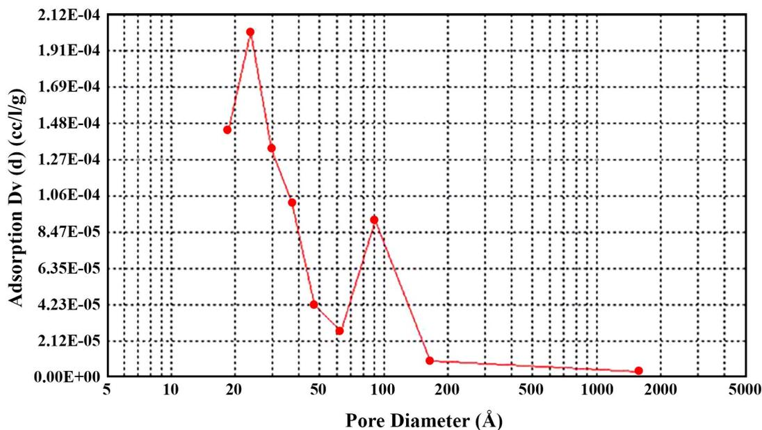
Fig. 4. The absorption curve (BJH) of hydroxyapatite sample.
