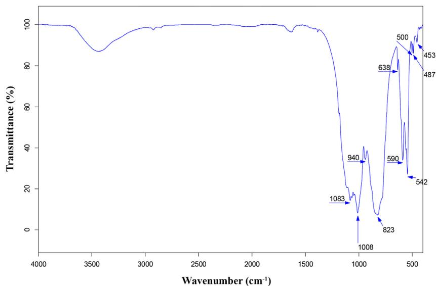
Fig. 5. Fourier transform infrared spectroscopy results related to hydroxyapatite.
