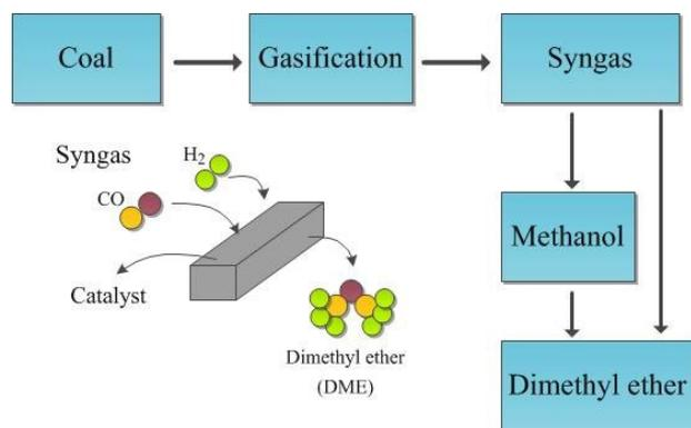
**Fig. 1.** Main chemical routes for syngas as feedstock to DME synthesis.
