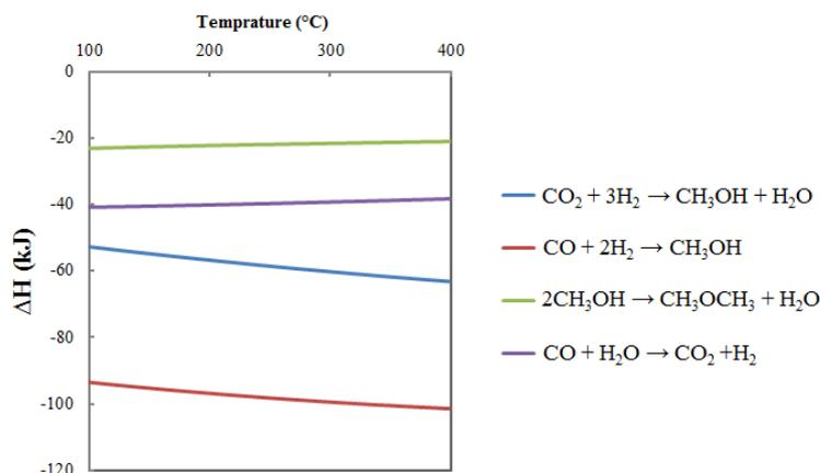
Fig. 2. Effect of temperature on the reactions during DME production.
