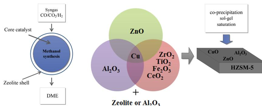
Fig. 4. Bifunctional catalysts and zeolite for direct synthesis of DME.
