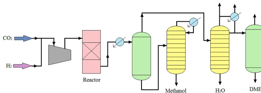
Fig. 3. The process scheme of direct synthesis of DME from CO<sub>2</sub> and H<sub>2</sub>.
