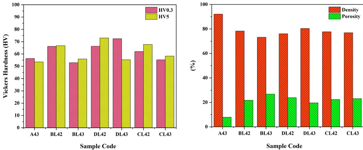
Fig. 5. The mechanical characteristic results of hot-pressed Zn-based nanocomposite samples.
