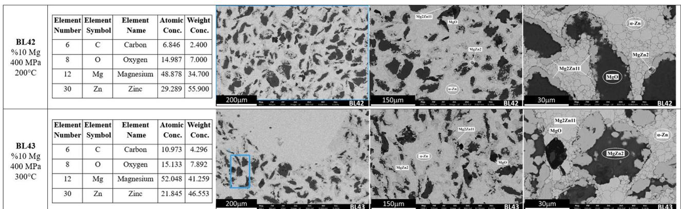
**Fig. 2.** The SEM micrographs and EDS analysis results of BL42 and BL43 samples with 10 wt% Mg content.
