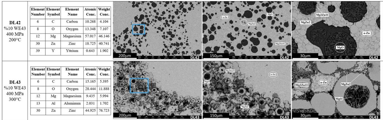
Fig. 3. The SEM micrographs and EDS analysis results of DL42 and DL43 samples reinforced with 10 wt% WE43 magnesium alloys powder.
