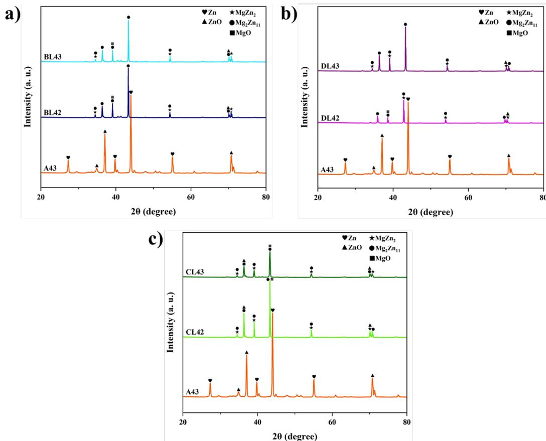
Fig. 6. a–c) The X-ray diffraction (XRD) analysis diagrams of Zn-based nanocomposite samples.
