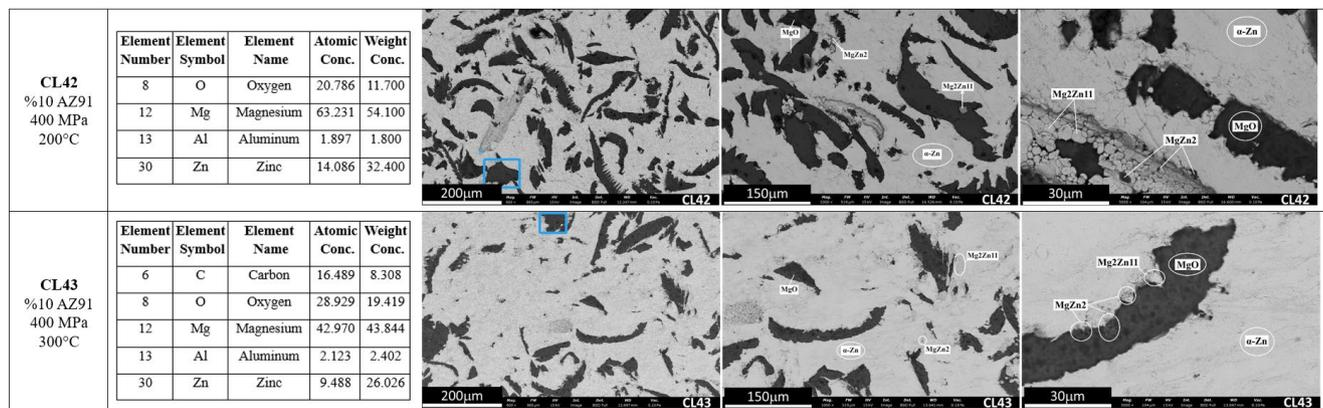
Fig. 4. The SEM micrographs and EDS analysis results of CL42 and CL43 samples containing 10 wt% AZ91 magnesium alloys powder.
