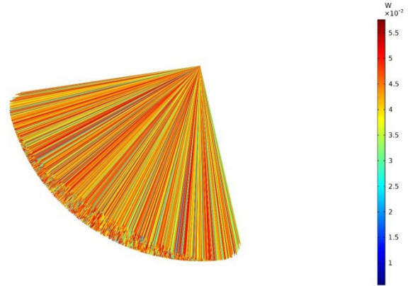
Fig. 3. The ray trajectories from the parabolic collector and concentration in the receiver surface.
