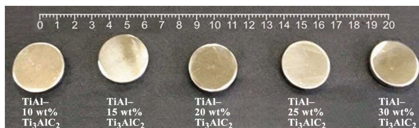
Fig. 3. Five spark plasma sintered TiAl-based samples with different amounts of \text{Ti}_3\text{AlC}_2 additives.
