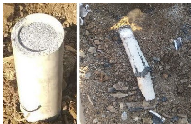
Fig. 1. Photograph showing cracking of an alumina tube mold due to thermal shock during thermite reaction.
