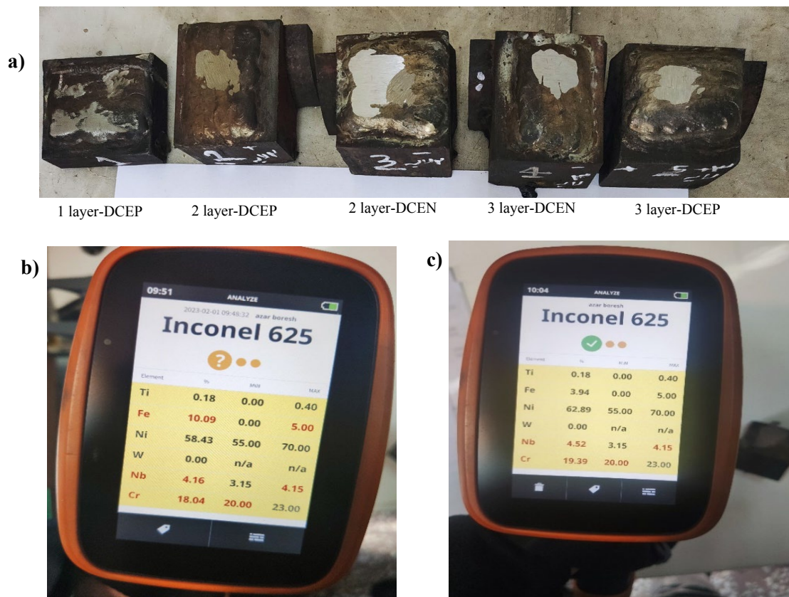
Fig. 1. a) Clad specimens prepared under various welding conditions and b & c) chemical composition measurements using a portable positive material identification (PMI) analyzer: b) Three-layer DCEP and c) three-layer DCEN.
