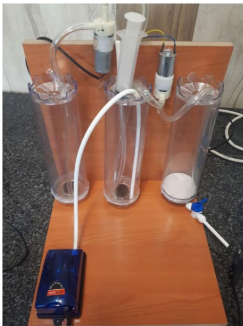
Fig. 10. Schematic representation of a device engineered for the filtration of chromium from industrial wastewater.
