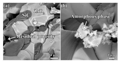
Fig. 3. SEM fractographs of pressureless sintered ZrB<sub>2</sub>-SiC composite doped with 1.5 wt% hBN.
