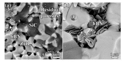
Fig. 5. SEM fractographs of pressureless sintered ZrB<sub>2</sub>-SiC composite doped with 4.5 wt% hBN.
