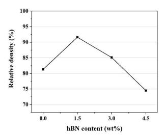
Fig. 1. Relative density of pressureless sintered ZrB<sub>2</sub>–SiC composites as a function of hBN content.
