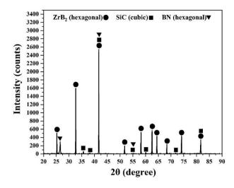
Fig. 2. Phase analysis of pressureless sintered ZrB<sub>2</sub>–SiC composite doped with 4.5 wt% hBN.
