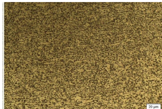
Fig. 7. Metallographic image of base metal. The bright matrix is \alpha -phase, and the dark region is \beta -phase.
