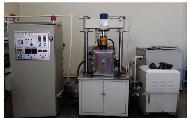
Fig. 4. The SPS apparatus used for the densification of pellets.
