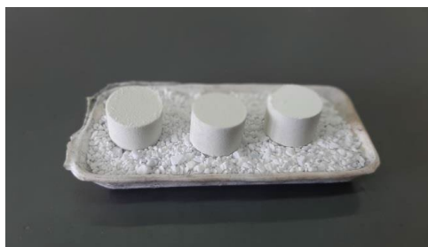
Fig. 2. Image of three representative cylindrical green body pellets prepared by uniaxial hydraulic pressing before sintering.
