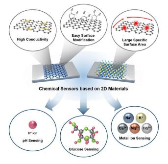
Fig. 2. A conceptual diagram illustrating chemical sensors that leverage 2D materials, highlighting the benefits of these materials and their use in detecting ions and molecules [37].
