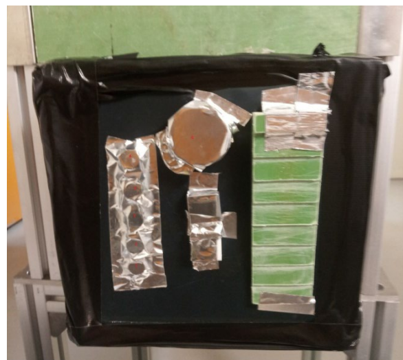
Fig. 1. Arrangement of Neutron radiography test. Left side: Al-30 wt% B 4 C; right side: PE-7% B.
