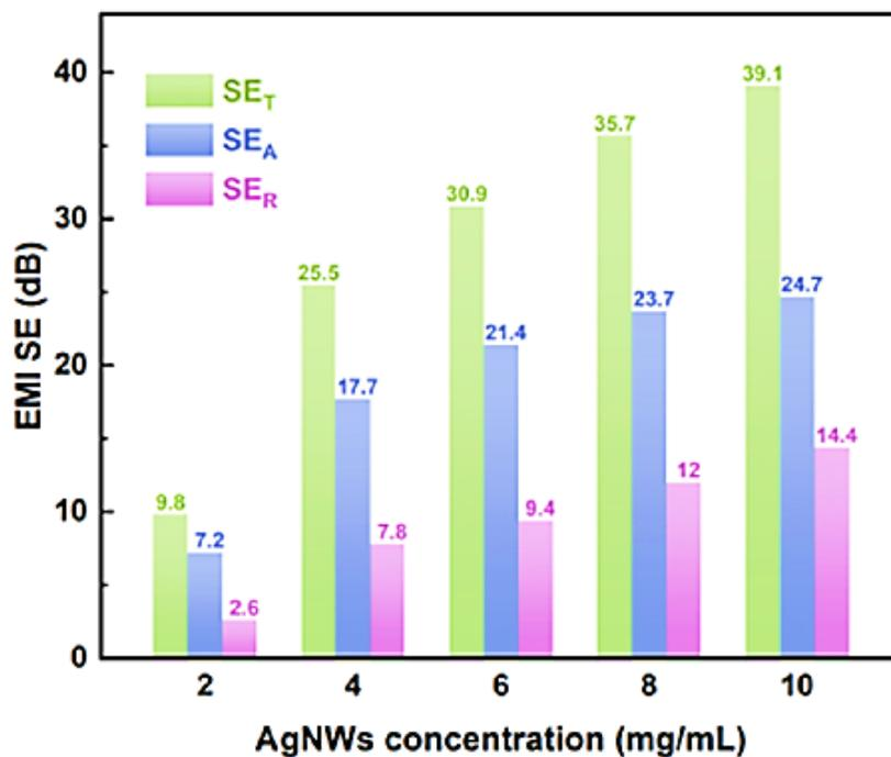
Fig. 18. Protective efficiency of samples coated with AgNWs in dB with different concentrations. With permission from Elsevier B. V. [86].
