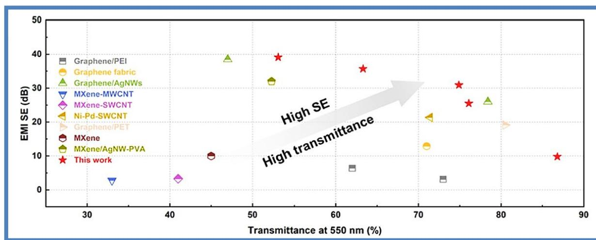
Fig. 20. SET was recorded for all samples in the X-band (8–12 GHz). Reprinted with permission from Ref. [86]. (Copyright 2024 American Chemical Society).
