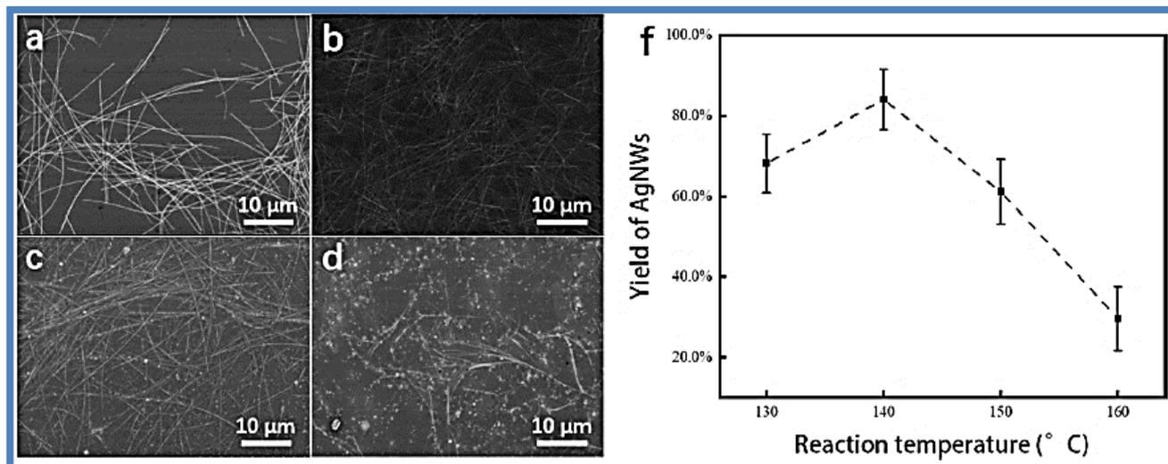
Fig. 10. SEM images of AgNWs obtained at different temperatures: a) 140 °C, b) 130 °C, c) 160 °C, d) 150 °C, and f) yield of AgNWs from different reaction temperatures. Reproduced with permission from Ref. [12].
