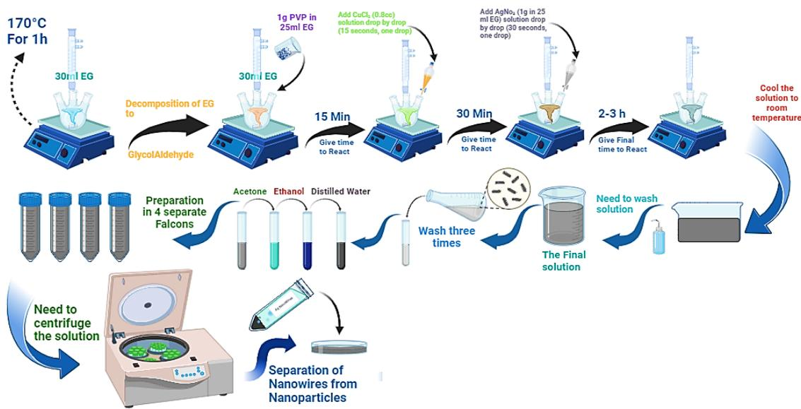
Fig. 3. Schematic from the synthesis of silver nanowires to their washing [1].
