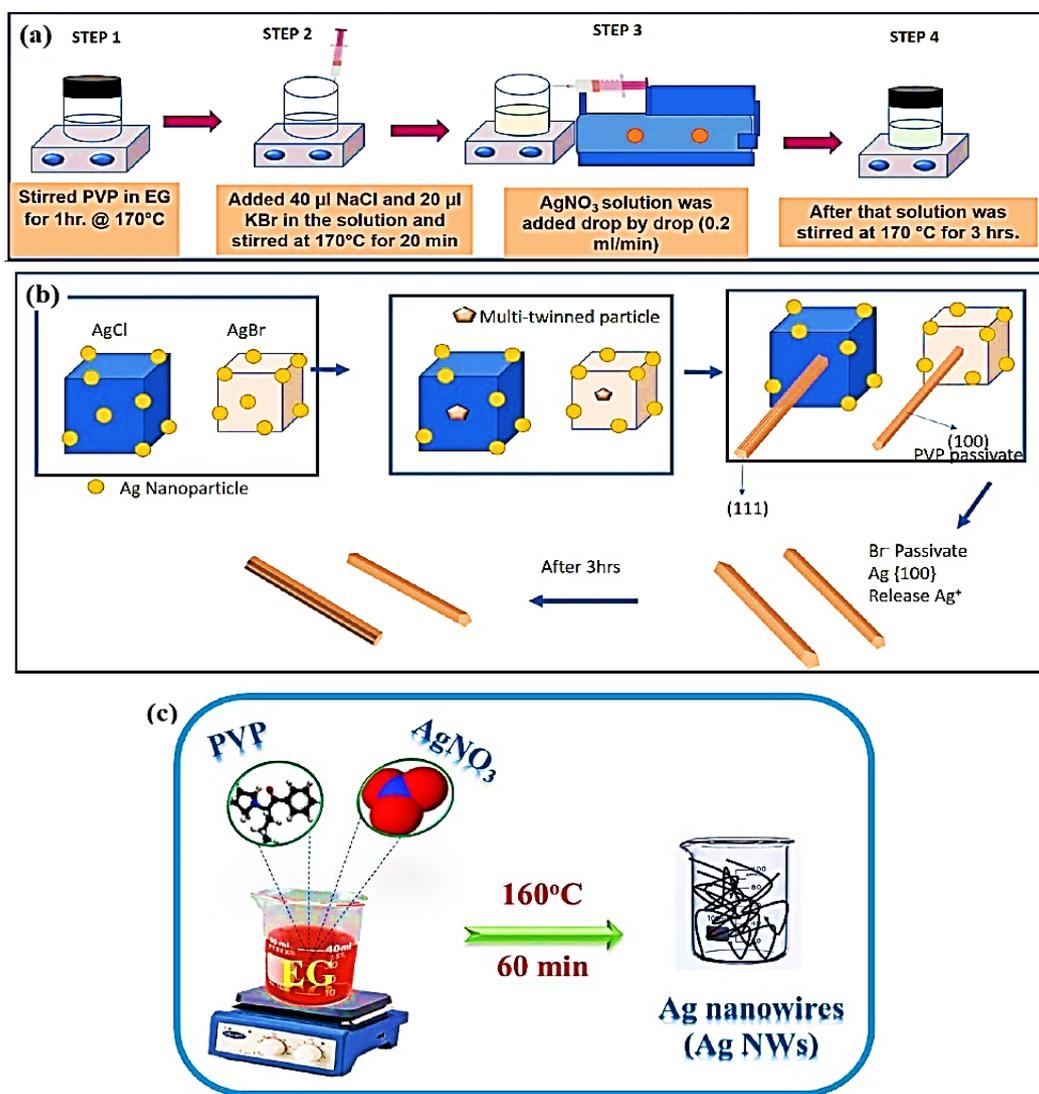
**Fig. 8.** a) Schematic of experimental process of the AgNWs synthesis, b) mechanism of silver nanowires growth [7], and c) Schematic illustration for the AgNWs synthesis [18]. Reproduced with permission from Refs. [7, 18].
