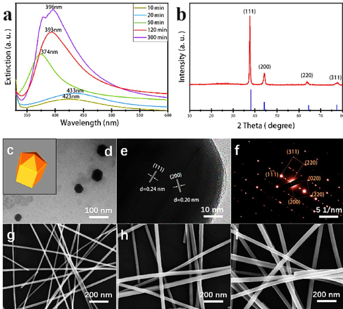
**Fig. 13.** a) UV-vis absorption spectra of AgNWs at different reaction stages, b) XRD spectrum of AgNWs, c) geometrical simulation graphics of quintuple twin nanoparticles, d) TEM image of nanoparticles obtained at 10 min reaction time, e) HRTEM image of AgNWs, f) SAED pattern of AgNWs, g–i) SEM images of AgNWs obtained at different times (g: 50 min, h: 120 min, and i: 300 min).
