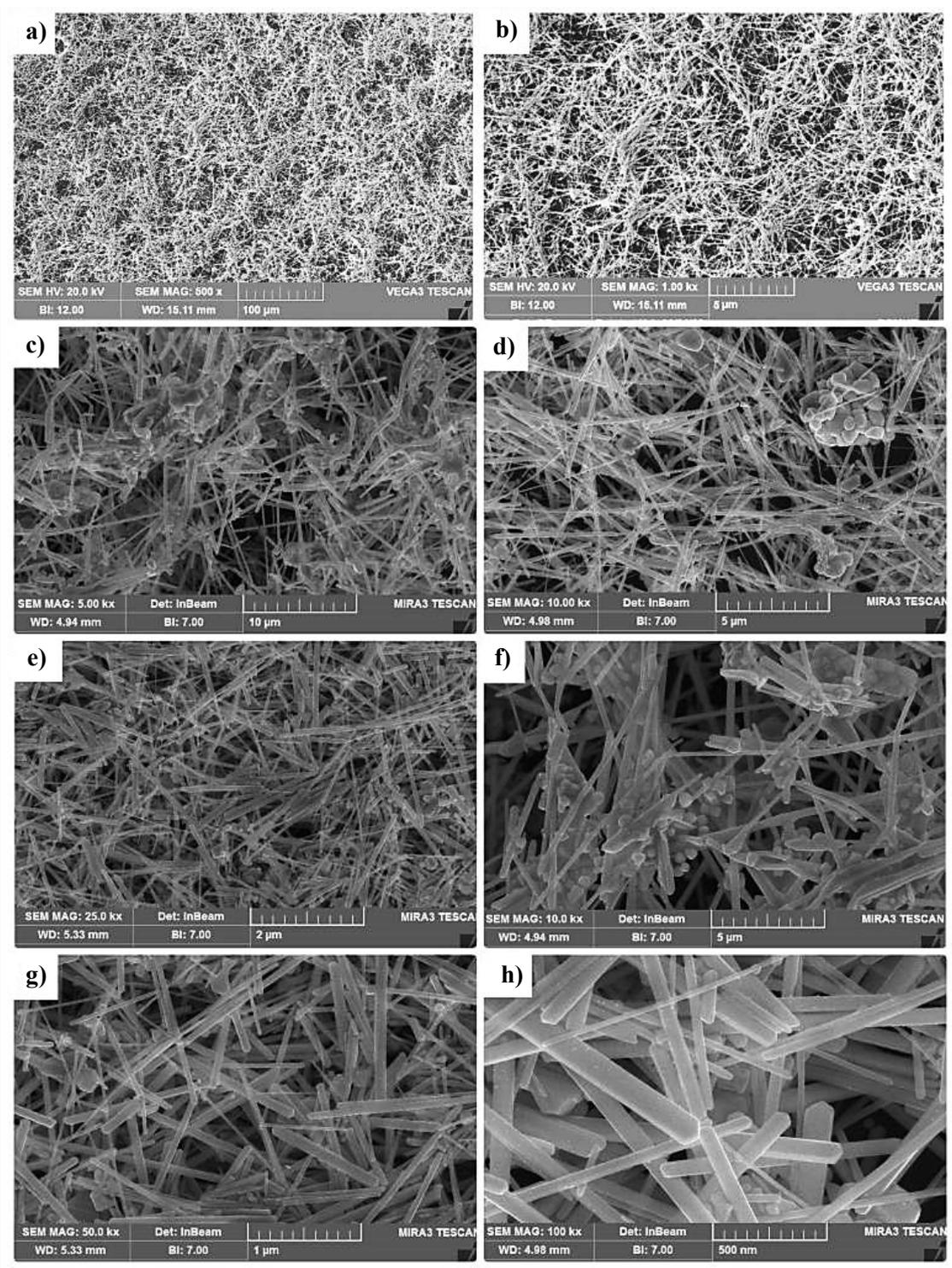
Fig. 15. a & b) SEM images and c–h) FE-SEM images of silver nanowires using different molar ratios [1].
