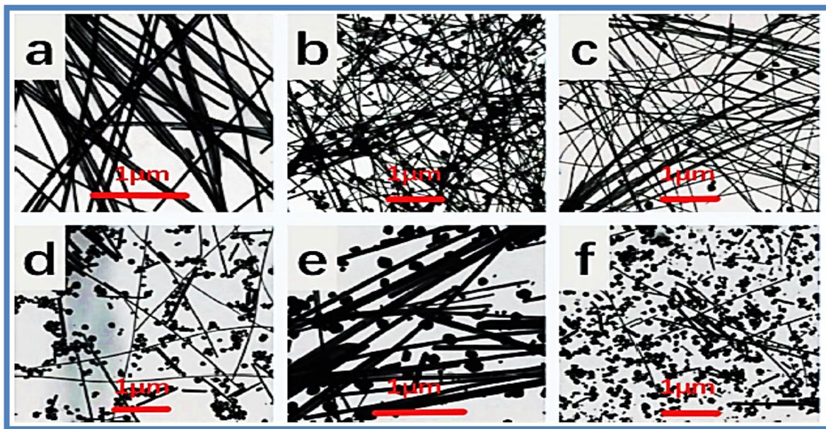
Fig. 12. TEM images of AgNWs synthesized using a) 0.125 mM NaCl, b) 0.1 mM NaCl, c) 0.025 mM KBr, d) 0.041 mM NaCl, e) 0.041 mM KBr, and f) 0.0840 mM KBr. Reproduced with permission from Ref. [67].
