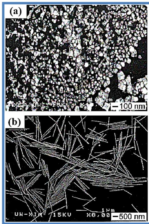
Fig. 9. SEM image of the product at a) 100 °C and b) 185 °C. Reproduced with permission from Ref. [16].
