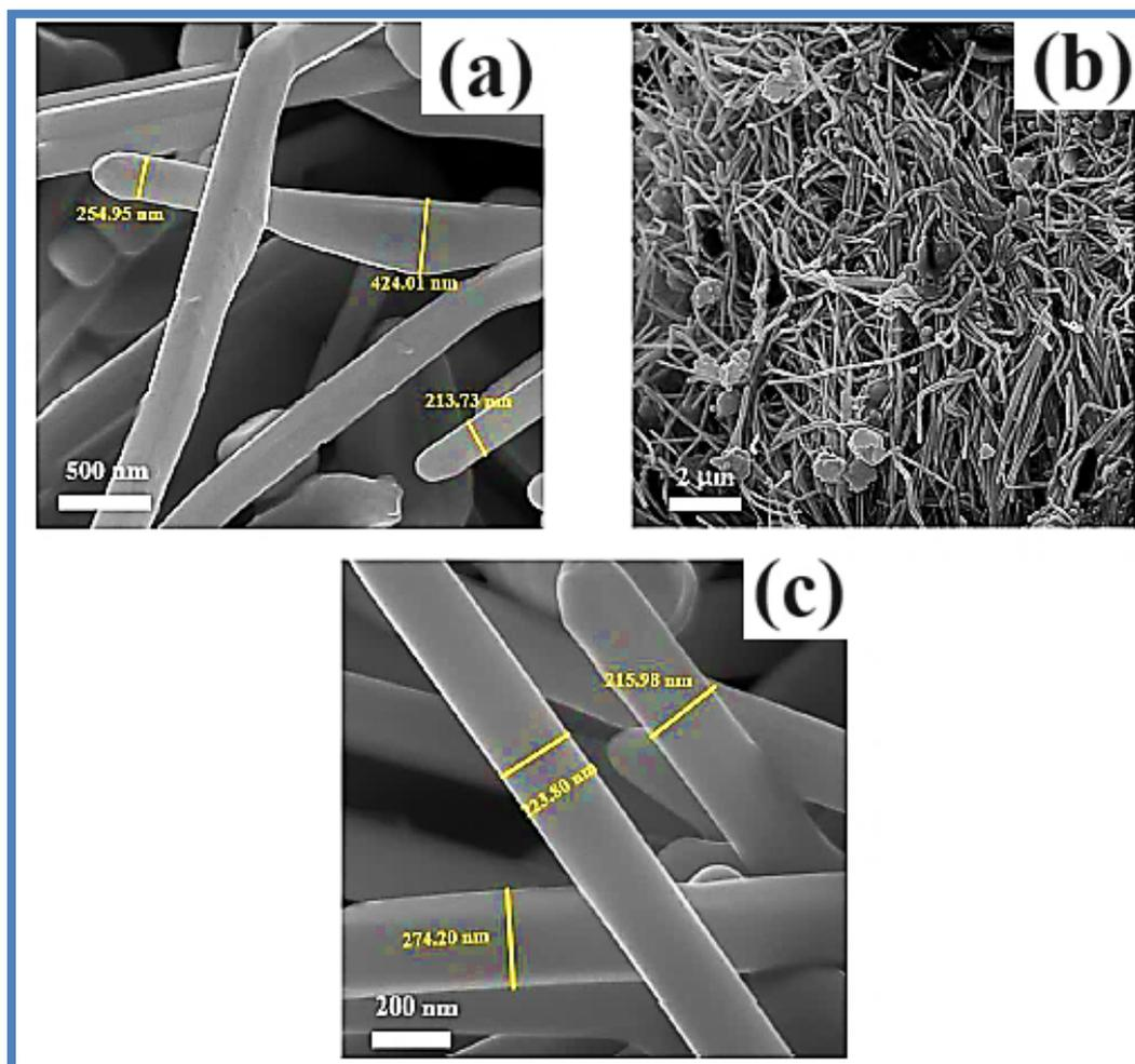
**Fig. 14.** FE-SEM images of silver nanostructures synthesized under different mixing rates at a) 300 rpm, b & c) 1200 rpm. Reproduced with permission. from Ref. [9].
