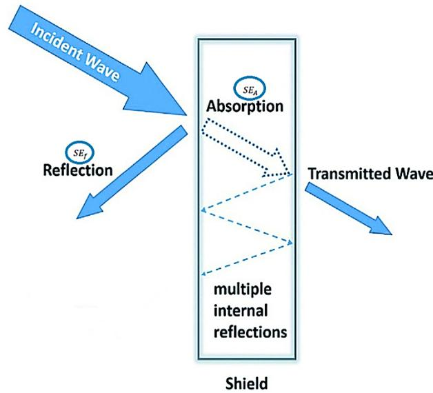
Fig. 17. EMI shielding mechanism. Reproduced with permission from Ref. [5].
