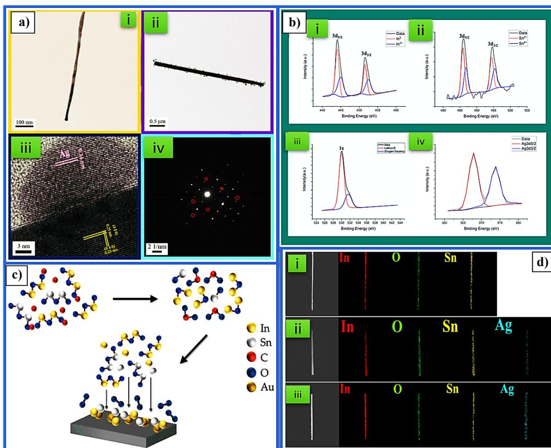
**Fig. 5.** a) i & ii: TEM images, iii: HR-TEM image of the Ag-ITO NW, and iv: SAED pattern, b) XPS interpretation of spectra for i: In, ii: Sn, iii: O, and iv: Ag, c) schematic presentation of the growth mechanism of ITO NW, where the reaction follows the VLS route, and d) EDS mapping of the: i) ITO NW, ii) 1 at% Ag-ITO NW, and iii) 3 at% Ag-ITO NW. Reproduced with permission from Ref. [11].
