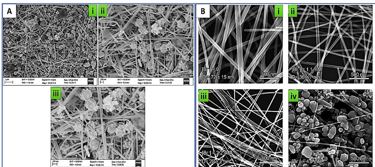
**Fig. 11.** a) FESEM images of silver nanostructures in NaCl concentration (10 mM) and b) high-resolution SEM images of the purified products obtained at different concentrations of: i) 0 mM NaBr, ii) 1.1 mM, iii) 2.2, and iv) 4.4 mM. Reproduced with permission from Refs. [13, 20].
