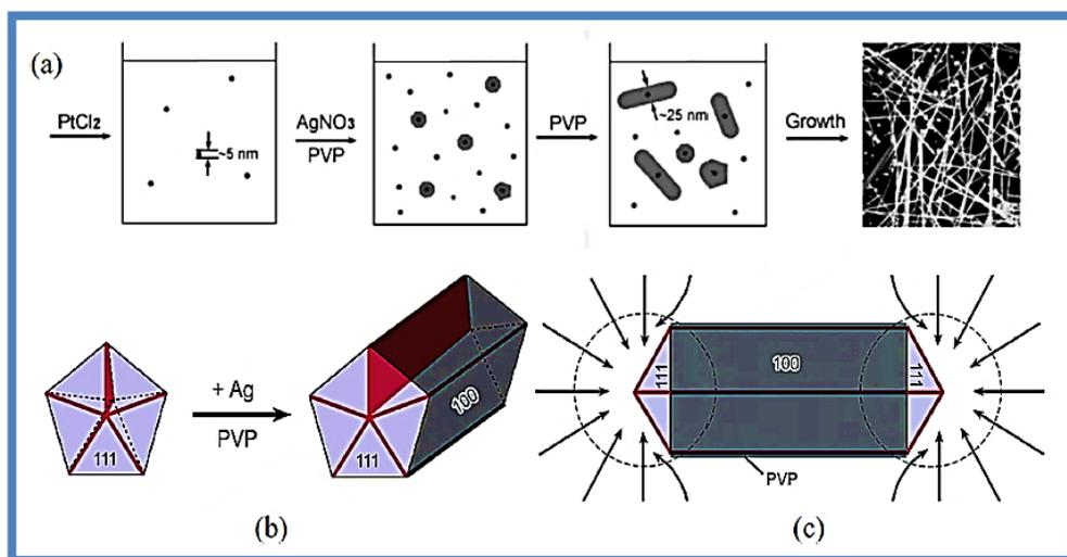
**Fig. 7.** a) Schematic illustrating the platinum seed polyol process's production of AgNWs [4], b) pentagonal section boundaries. PVP passivated the sidewalls of the nanorods after, and c) dispersed silver atoms to both of their ends [16]. Reproduced with permission from Refs. [4, 16].
