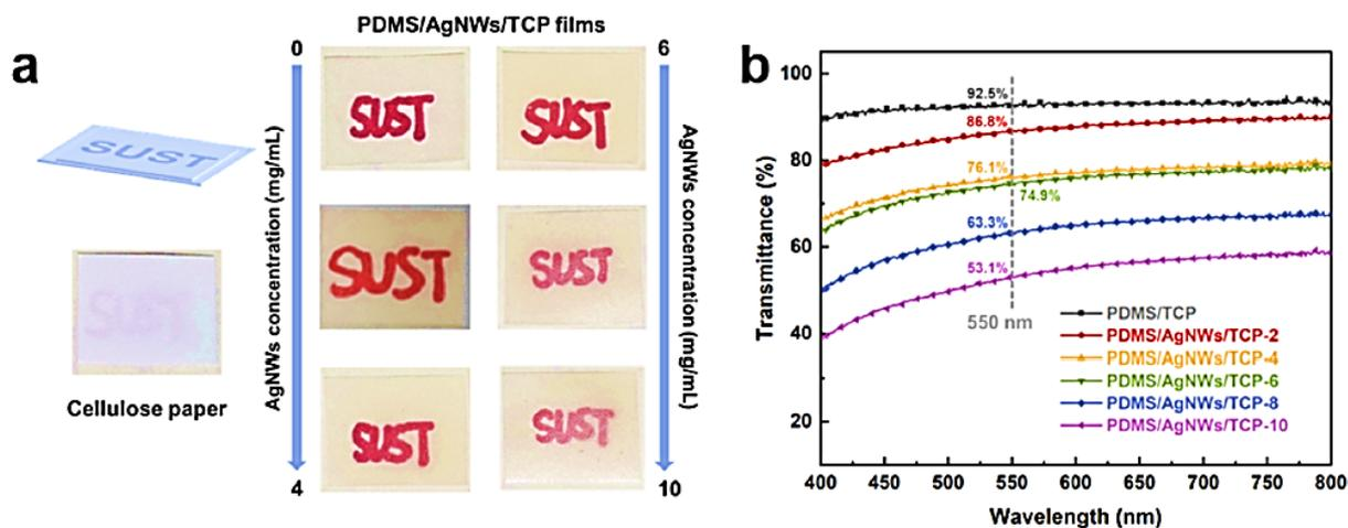
Fig. 16. a) Transparency of light transmission spectrum of six samples coated with silver nanowires and b) coated glass samples.
