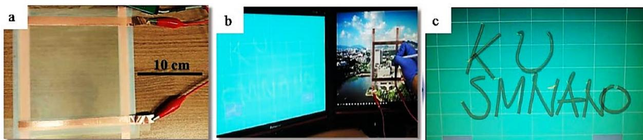
**Fig. 19.** a) AgNW-SiO<sub>2</sub>-based touch panel, b) writing on the touch panel, and c) letters written. Reprinted with permission from Ref. [8].
