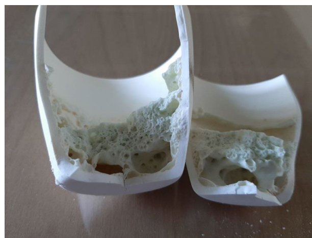
Fig. 2. One of the ceramic crucibles including synthesized powder removed from the furnace.
