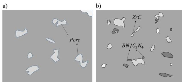
Fig. 2. The schematic representation of the polished surfaces of a) ZrB<sub>2</sub> and b) C<sub>3</sub>N<sub>4</sub>-doped ZrB<sub>2</sub> ceramics [9].
