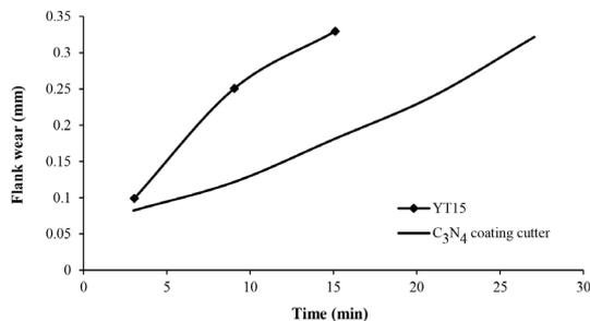
**Fig. 3.** The tool flank wear-time curve under the condition:  $V_c = 60$  m/min,  $f = 0.1$  mm/r, and  $ap = 0.4$  mm [36].
