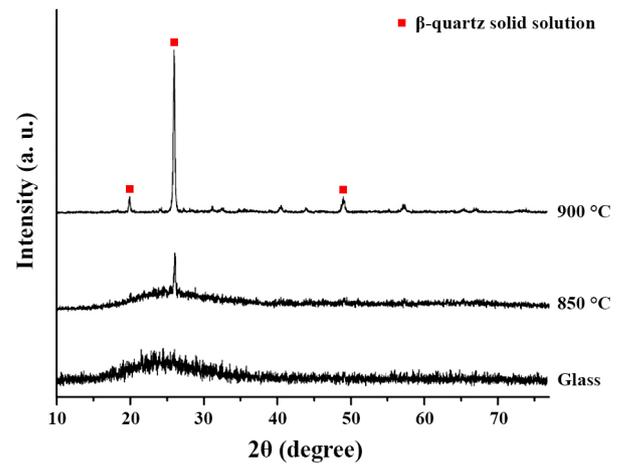
Fig. 6. XRD patterns of the glass powder and the samples heat treated at 850 and 900 °C for 1 h.
