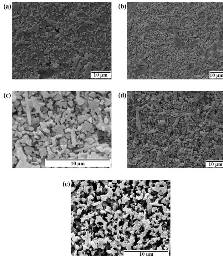
**Fig. 11.** SEM micrographs of the samples heat-treated through a) one-step, b) two-step, c, d) three-step sintering procedures, and e) the bulk sample.
