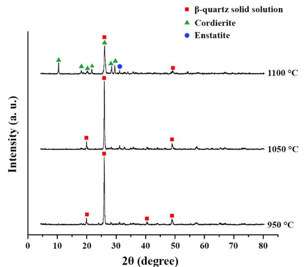
Fig. 7. XRD patterns of the samples heat treated at 950, 1050, and 1100 °C for 1 h.
