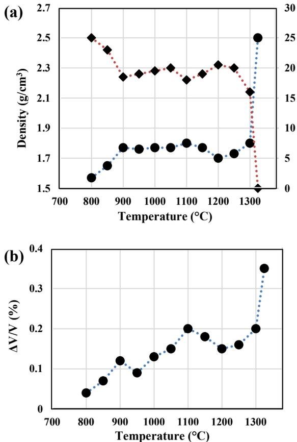
Fig. 5. Sinterability parameters versus one-step sintering temperature, a) density and water adsorption and b) shrinkage.
