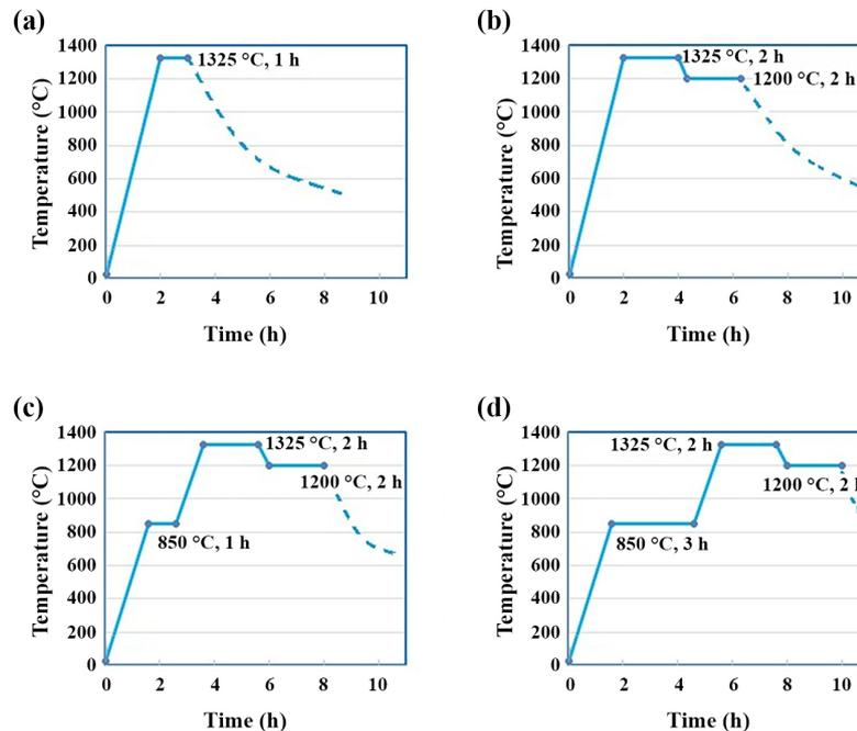
Fig. 2. Heat treatment schedules of glass powders: a) one-step, b) two-step, and c, d) three-step sintering.
