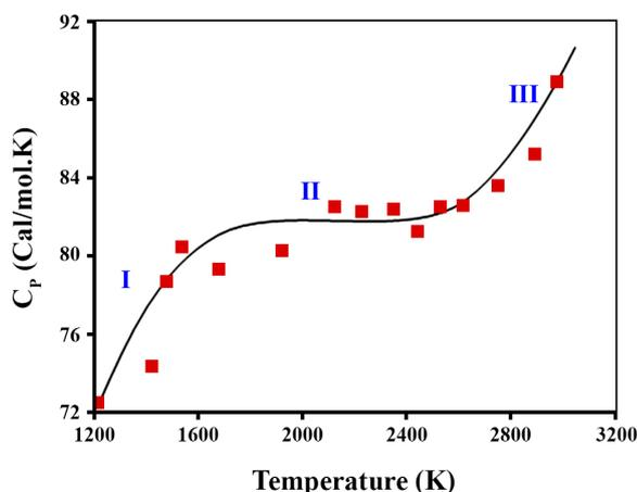
Fig. 1 Average heat capacity of zirconium dioxide versus temperature.
